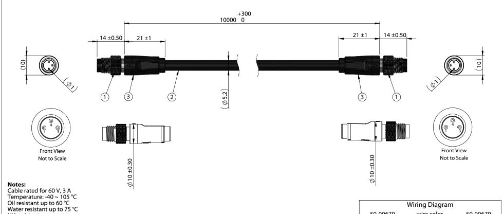
IP67 waterproof rating when mated with corresponding (IP67) connector
